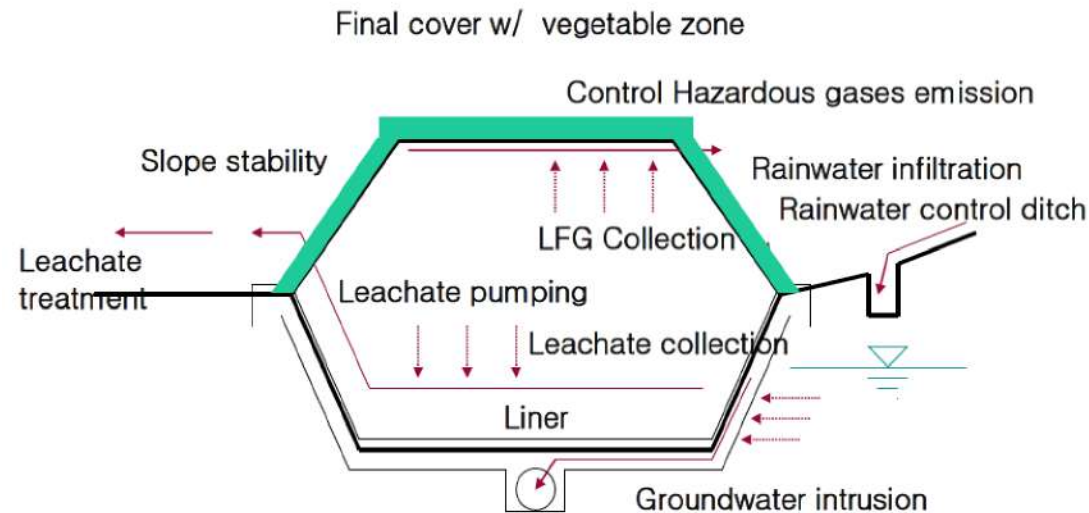
Cross section of a typical engineered landfill
