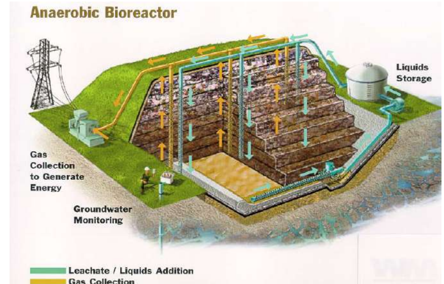
Source: Don Davies Stantec Consulting Ltd.; 2010; Sustainable landfill biocell
