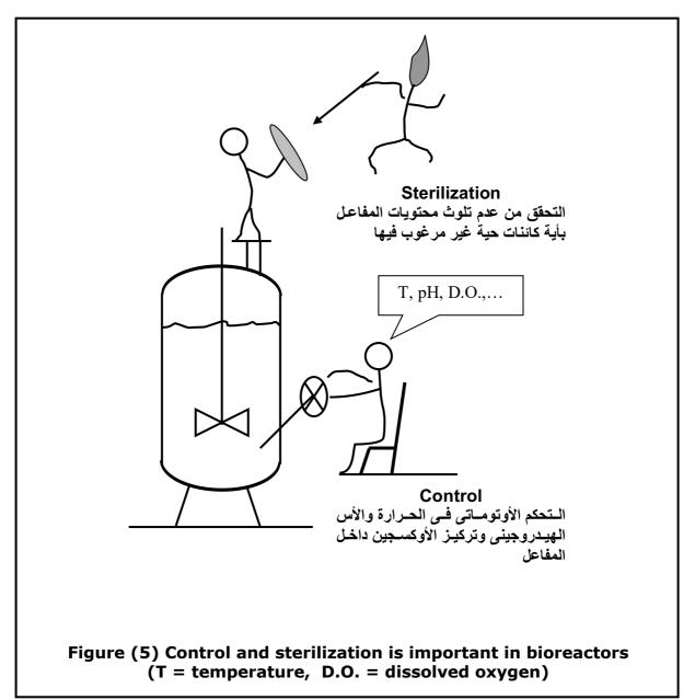
A principal task in the operation of bioreactors is the prevention of contamination by surrounding microorganisms. The inside of a bioreactor is designed to be suitable for microorganisms to grow, so those foreign microorganisms with high growth rates will grow rapidly while the desired microorganisms or cells may die. Careful sterilization of the equipment an feedstocks is therefore essential.
