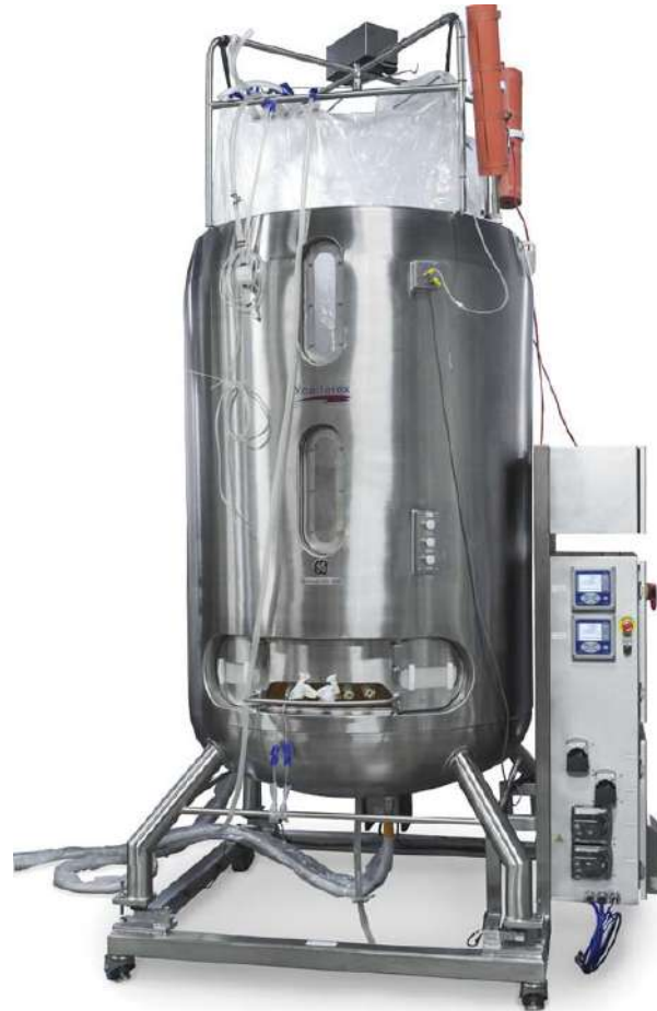
2000 L bioreactor with disposable bag
