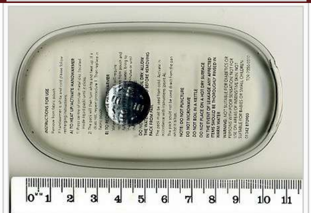
Crystallisation-type hand warmer with scale showing metal disc trigger
