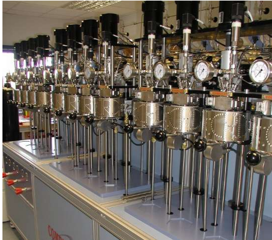
Figure 7 An example showing some pilot batch reactors which are separate and operate in parallel. A computer controls each one and users can perform series of experiments, changing temperature, pressure and catalyst composition.
