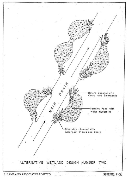
6) The return segments will be designed such that when the water is returned to the main drain, a moderate mixing with mild turbulence is created to produce aeration and coagulation of suspended particulates.
